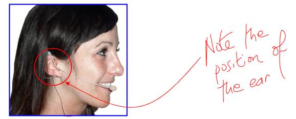
Flex or bend carefully (without breaking it!) the microphone boom, to perfectly fit the shape of your face. Take your time flexing and bending to find the most comfortable and suitable position of the device for you; as it is made out of titanium alloy!...
