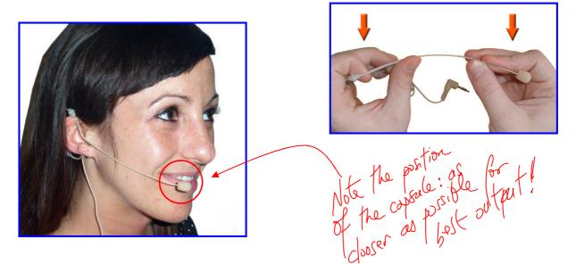
d) Connect the gold, non corrosive, audio jack of the *FlexyMike*<sup>TM</sup> to your PC Soundcard microphone port. This port is normally colored red. Push it to make perfect contact. Optionally, to avoid popping and background noise, use the windshield included in the box.
